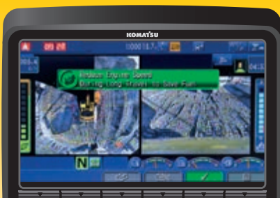
Eco-gauge, Eco guidance and fuel consumption gauge
