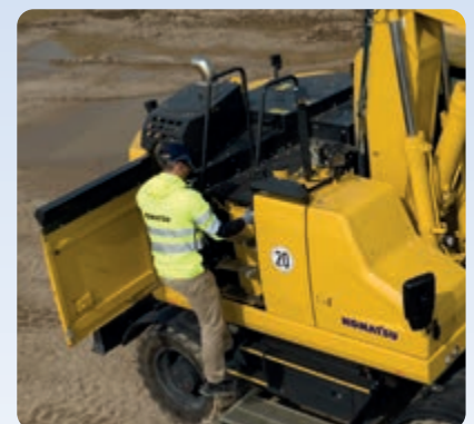
Handrails and anti-slip plates for convenient and safe maintenance access
