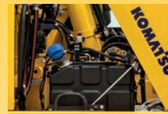
Simple access to the AdBlue® tank
