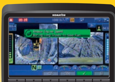
Eco-gauge, Eco guidance and fuel consumption gauge
